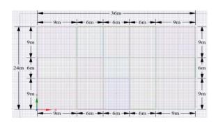
Fig.1 Plan of half breed wood steel building
