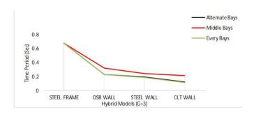
Fig. 3. Timespan of (G+3) Hybrid Buildings
